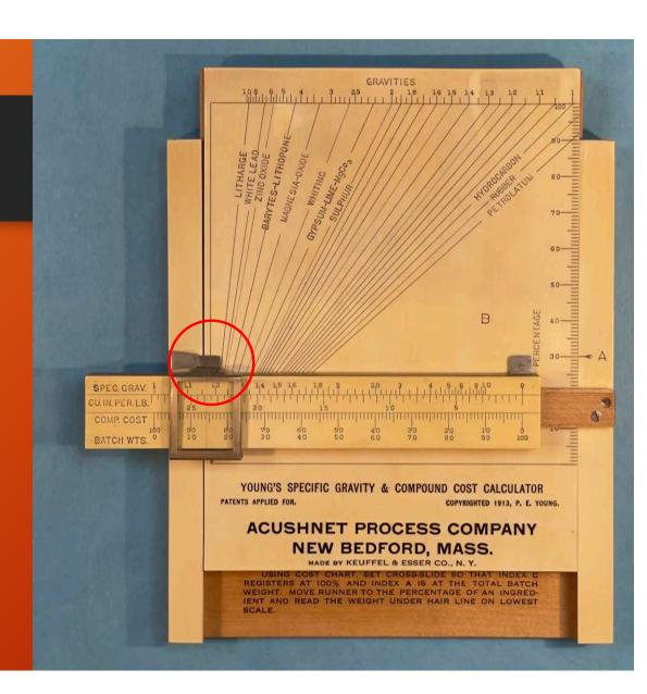
Read the Specific Gravity under the hairline position on the upper SPEC. GRAV. scale
